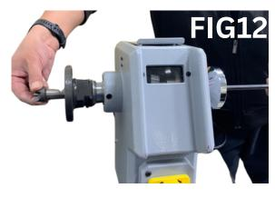
2. To re-insert the drive center, place it in the hole in the faceplate, and while using a block of wood and a hammer, tap the drive center to "set" it in the headstock.
