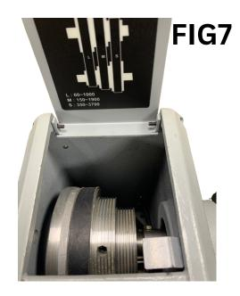
2. To expose the motor pulleys, open the motor access door by graping the knob and pulling it outwards. SEE FIG 8 & 9
